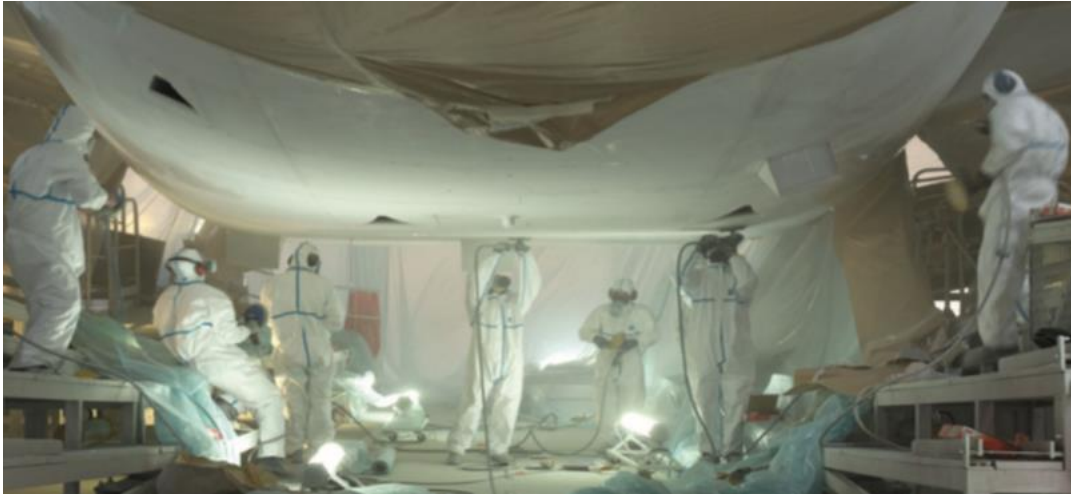
Figure 1.2: Stripping of the bottom part of the airplane manually.
