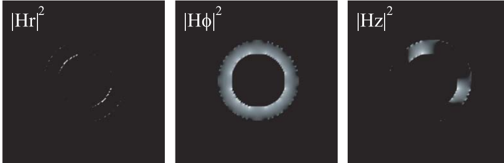
FIGURE 5 Square modulus of the three cylindrical components of the magnetic field in the case of the TEM mode of Fig. 8 ( \lambda = 528 nm and k_z = \frac{2\pi}{500} nm ^{-1} )
